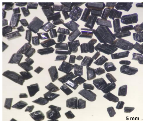
Figure 1. Allanite grains as viewed under a stereomicroscope at \sim 20\times magnification.
