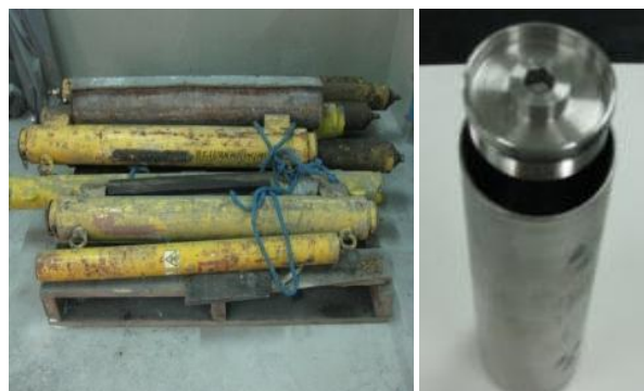
Figure 1. Category 3-5 Sources and a stainless steel capsule used in conditioning.
