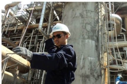
Denis Aquino, Senior Science Research Specialist of Isotopes Techniques Section, performs gamma-ray scanning during a training course in a petro-chemical plant.
