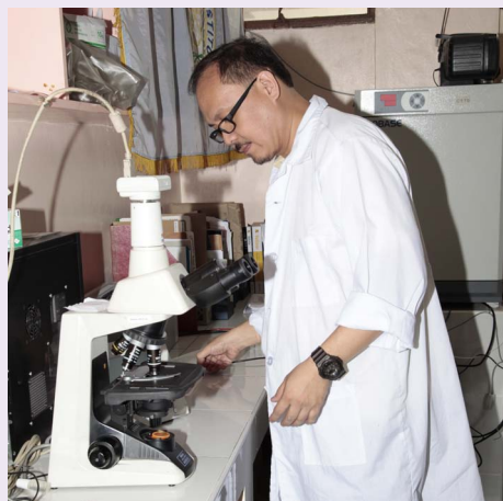
A PNRI researcher (left) observes blood samples through a microscope for dicentric chromosomes (right) which will be used to determine the radiation dose absorbed by a worker occupationally exposed to radiation.
