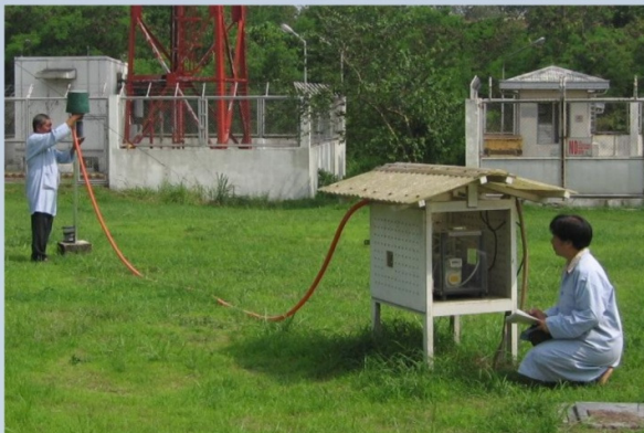
Left Photo: Gent sampler set-up at an air monitoring station
