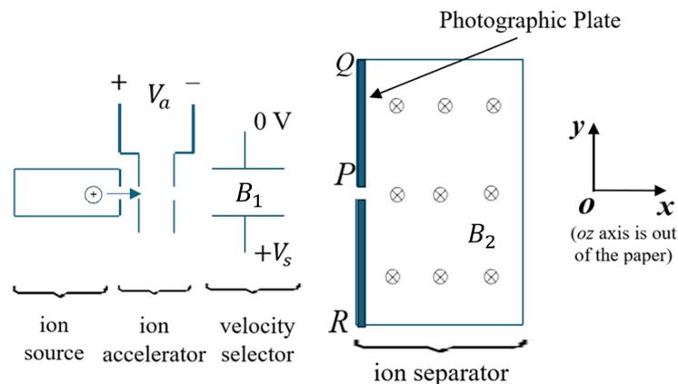
**Figure 1.** Schematic diagram of mass spectrograph
