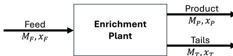
**Figure 1.** Material flow in an enrichment plant.
