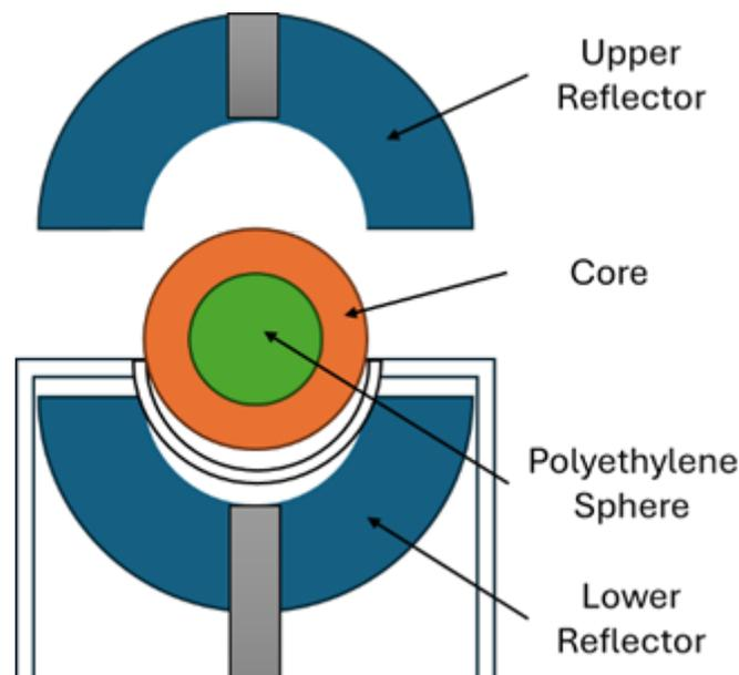
**Figure 2.** Approximate accident configuration of the FKBN assembly.
