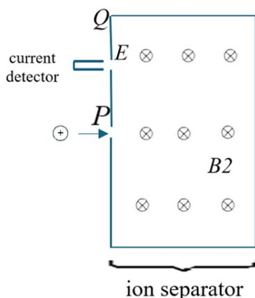
**Figure 2.** Ion separator for a mass spectrometer
