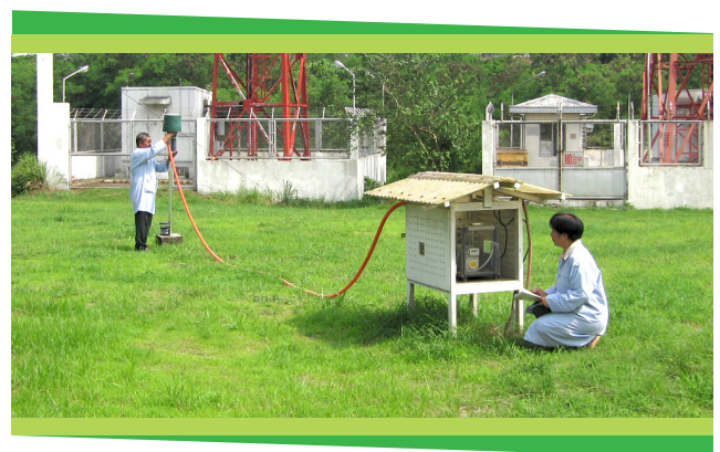
Gent Sampler set-up at an air monitoring station
