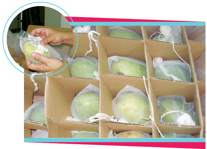
Researchers attached dosimeters on the mangoes to determine the radiation dose absorbed
