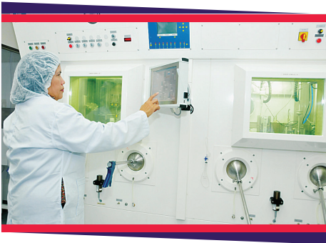
The Tc-99m hot cell facility inside the Radioisotope Laboratory building
