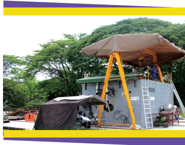
An assembled mobile hot cell for conditioning Spent High Activity Radioactive Sources
