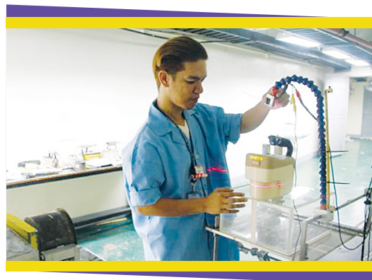
Calibration of a survey meter in the Secondary Standards Dosimetry Laboratory
