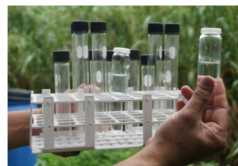
Air moisture collection for 18 O isotope analysis used in evapotranspiration measurements
