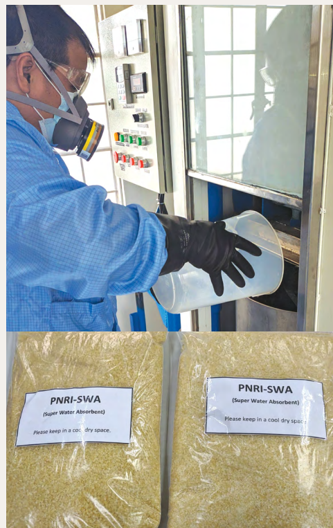
Pilot-scale production of SWA: Addition of acrylic acid to gelatinized starch
