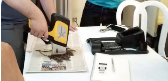
Analysis using PNRI's handheld XRF showed prominent copper and iron concentrations in fern root samples.
