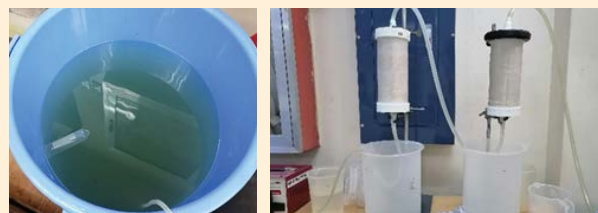
Wastewater being treated using the PNRI-developed adsorbent.
