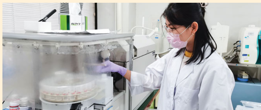
Laboratory experimentation in MALT-UTokyo: Left: Loading sample and calibration solutions in the automatic sampler of the Agilent ICP-MS 5700a. Right: Mixing Niobium (Nb) powder to the Silver Iodide (AgI) precipitate.
