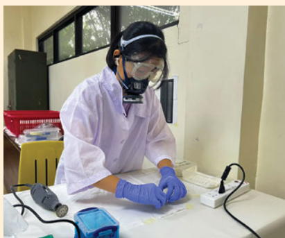
Manual subsampling of the WPS coral core 1 using Dremel® 3000 variable speed rotary tool fitted with a diamond wheel drill bit.
