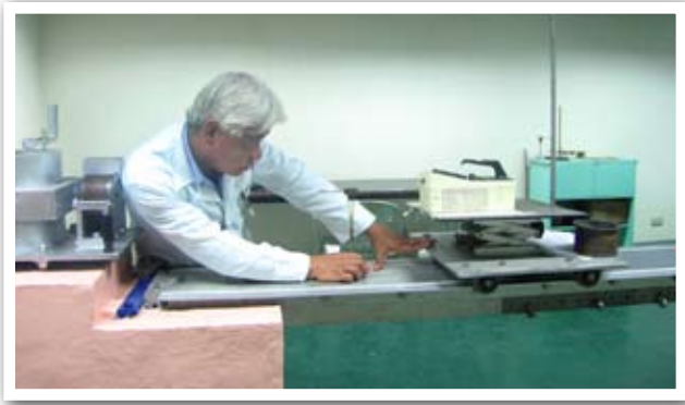
CALIBRATION OF A RADIATION MONITORING INSTRUMENT USING CESIUM-137 REFERENCE SOURCE AT THE SECONDARY STANDARDS DOSIMETRY LABORATORY
