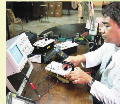
Repair of a radiation detection instrument
