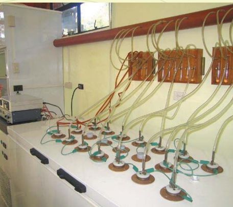
Electrolytic enrichment of tritium in water samples prior to liquid scintillation counting
