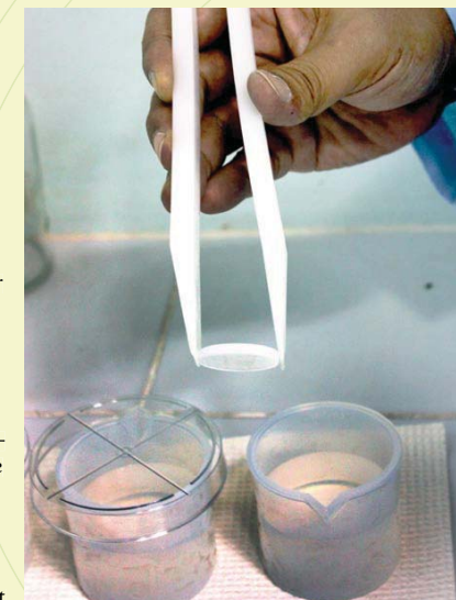
Quartz disc preparation for research study on metal adsorption properties of advanced materials
