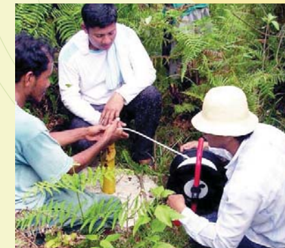
Inspection of the status of groundwater observation wells in the vicinity of the footprint
