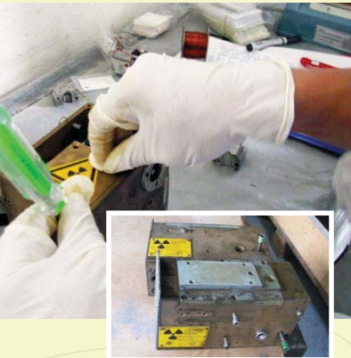
Removal of radiation source disposed from a nuclear density gauge from a cigarette factory
