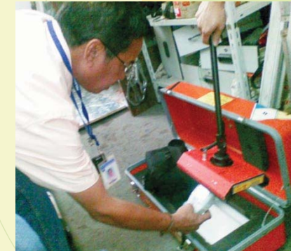
Monitoring and verification inspection of moisture density gauge containing Am-241 sealed source during regulatory inspection.
