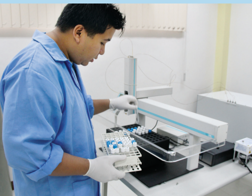
Analysis of ^{18}\text{O} and ^2\text{H} in water samples using Isotope Ratio Mass Spectrometry.
