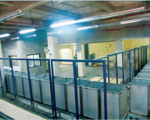
The new storage transfer system of the irradiator inside the Multipurpose Irradiation Facility at PNRI.
