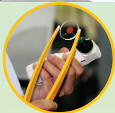
Heavy metals adsorbed in silica glass (inset) are analyzed for trace element using total x-ray fluorescence spectrometry.
