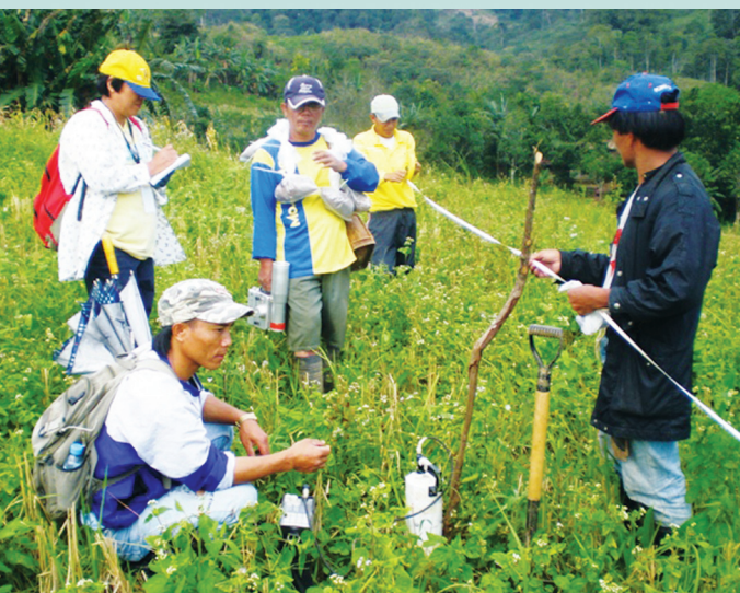
Collection of soil samples at Didipio, Nueva Viscaya for multi-element analysis at PNRI and in-situ measurement of potassium, uranium, thorium using gamma ray spectrometer.
