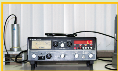
Participants in the training course for high school and college faculty perform an experiment using a Geiger Muller counter.
