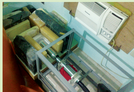
Set-up of the prompt-gamma neutron activation analysis facility consisting of a neutron source, sample chamber and high purity germanium detector.
