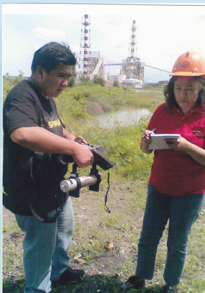
Ambient gamma dose rate measurement at the coal-fired power plant in Calaca, Batangas
