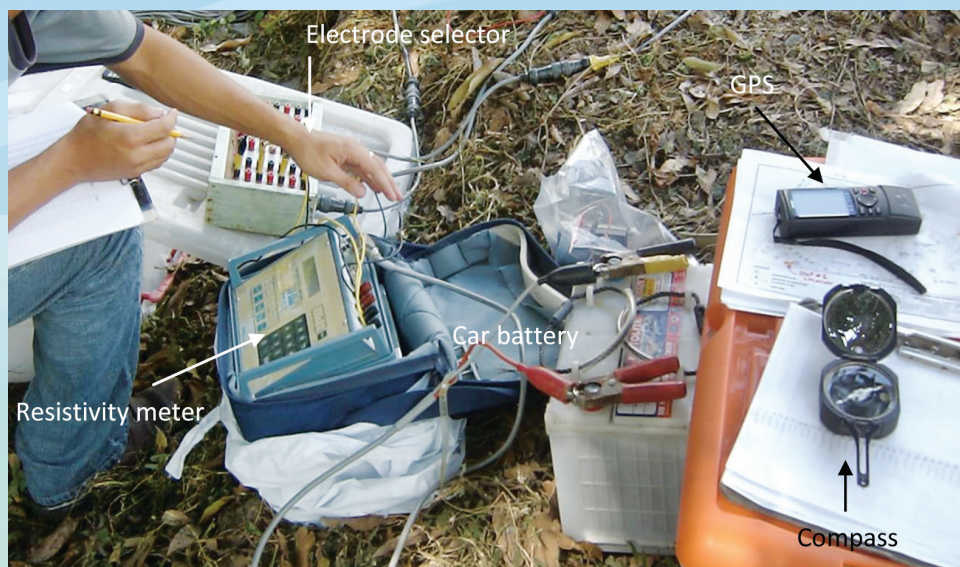
A set of instruments used in the field survey for geotechnical investigation and groundwater prospecting
