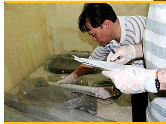
Verification of fuel at the spent fuel pool storage and fresh fuel storage of the Philippine Research Reactor-1
