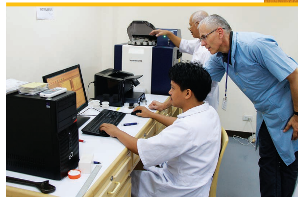
IAEA Expert Denis Topolavac trains NMRS staff in the use of Wavelength Dispersive X-ray Fluorescence Spectrometer (WDXRF) systems for characterization of rare earth elements.
