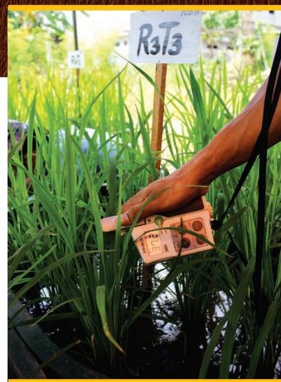
Measurement of chlorophyll content in rice plants using a portable chlorophyll meter as part of nutrient dynamic assessment of rice-based systems
