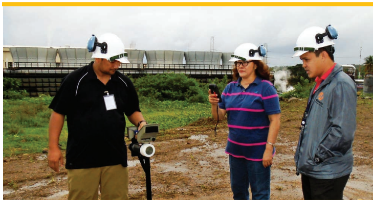
Ambient gamma radiation measurements around a geothermal power plant site as part of the project on the radiological assessment of NORM-TENORM
