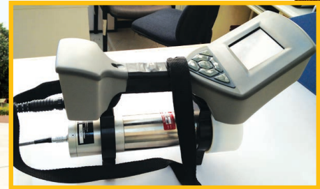
The Health Physics Research Section monitoring team conducts ambient gamma radiation monitoring in PNRI grounds using (inset) SAM-940 portable gammameter.
