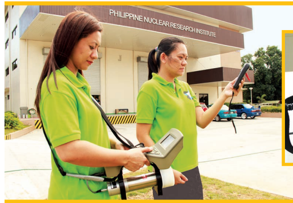
The Health Physics Research Section monitoring team conducts ambient gamma radiation monitoring in PNRI grounds using (inset) SAM-940 portable gammameter.
