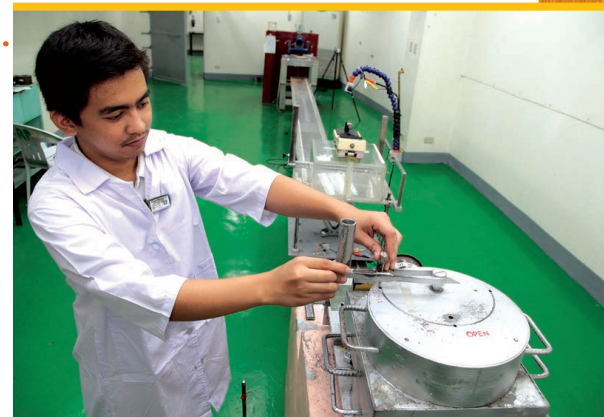
Calibration of a radiation survey meter at the PNRI Secondary Standards Dosimetry Laboratory
