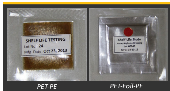
(Left) Honey alginate wound dressing in two different packaging materials for extended shelf-life study
