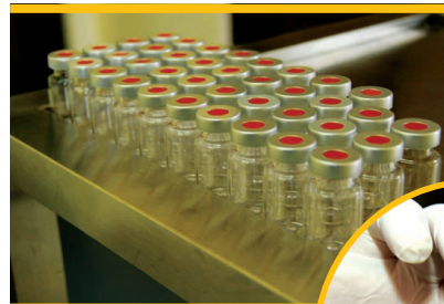
The cold kit formulations for synthesis of technetium-99m radiopharmaceuticals
