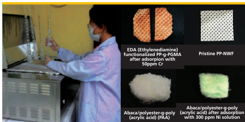
PNRI researcher preparing grafted material through radiation-induced chemical reaction
