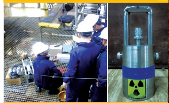
New radiation source holder for gamma column scanning
