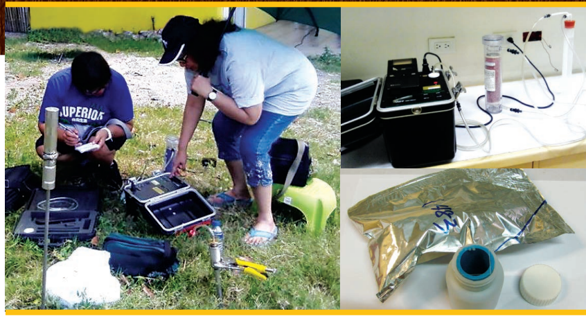
(Left) Radon measurement in soil gas and water using the portable electronic-based Durridge radon detector (Right) Passive Alpha Track etch CR39 detector and processing of CR39 films
