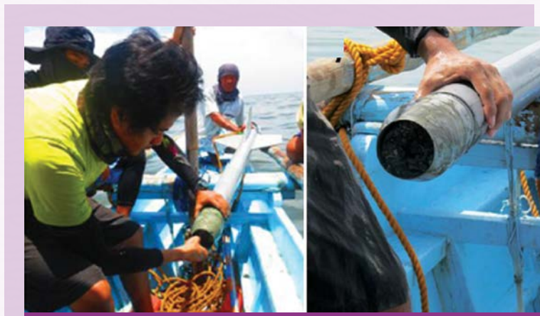
Collection of sediment cores in Manila Bay using a gravity corer Photo credit : Dr. Fernando Siringan (UP-MSI)
