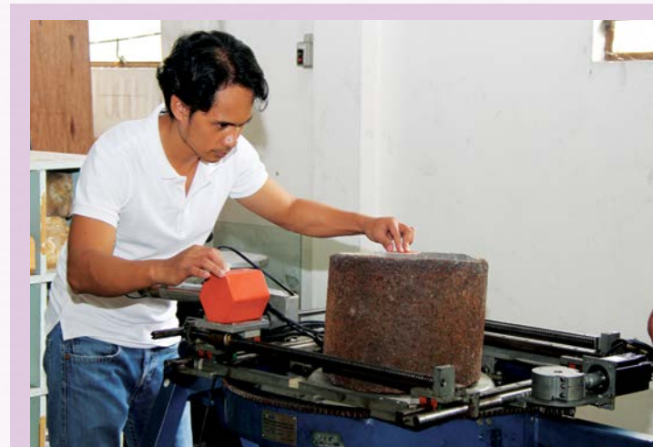
A PNRI researcher sets up the equipment for experiments on gamma computed tomography.
