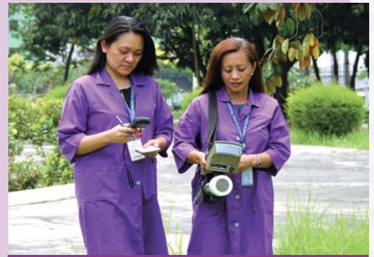
Ambient gamma radiation monitoring in PNRI grounds using SAM-940 portable gamma meter
