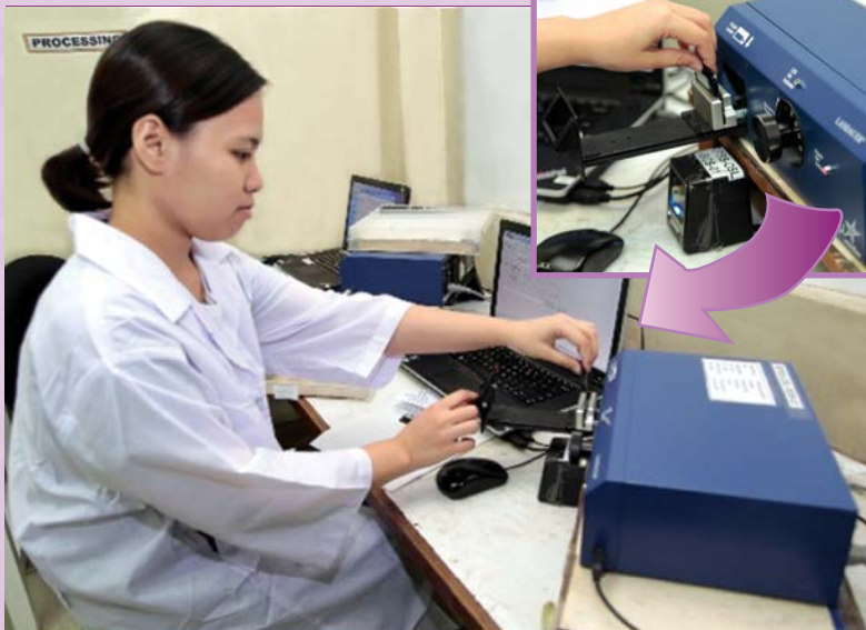
Analysis of radiation dose from an Optically Stimulated Luminescence (OSL) dosimeter of a worker occupationally exposed to radiation
