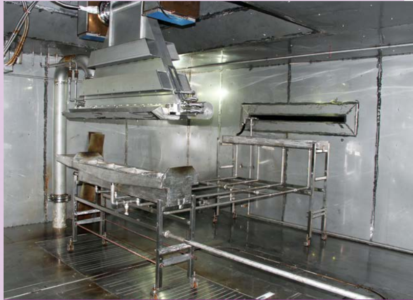
The electron beam scanning horn with the fabricated liquid handling system designed by EBIF personnel
