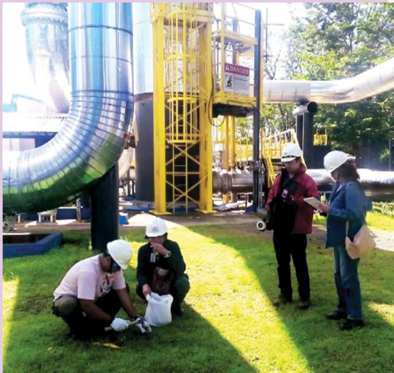
Radiation dose rate measurements and soil sampling at SS3 station of Philippine Geothermal Production Plant in Bay, Laguna
