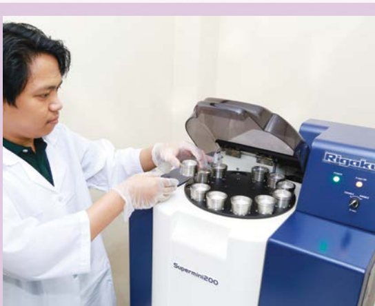
A PNRI researcher conducts elemental bulk analysis using X-ray fluorescence spectrometry.
