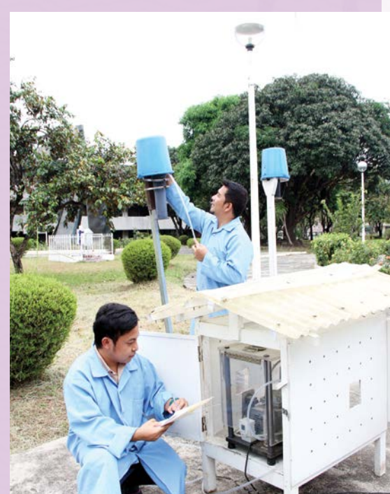
Air sample collection for air pollution studies at PNRI using Gent samplers
