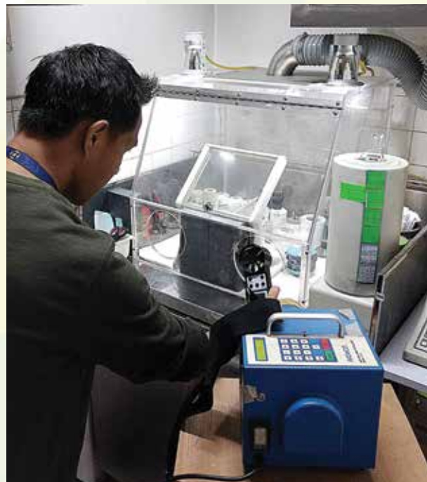
PNRI researcher conducts an assessment of the fume hood operation in a nuclear medicine facility
