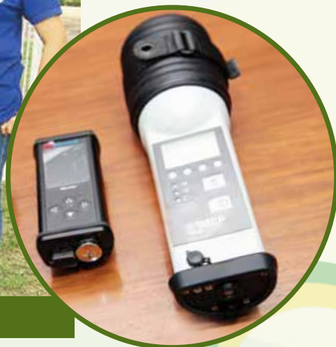
Monitoring in PNRI ground and its perimeter using a portable gamma dose rate meter (inset)
