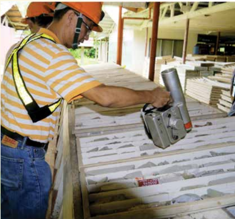
PNRI geologist scans core samples from Boyongan and Bayugo boreholes of Silangan Mindanao Mining Company, Inc. at Brgy. Timamana, Tubod, Surigao Del Norte for identification of elevated radioactivity in the layers of rock.
