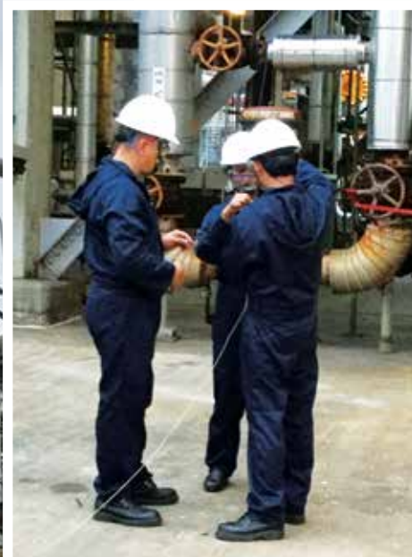
PNRI performs gamma column scanning to test the operating conditions of a distillation column in a refinery.
