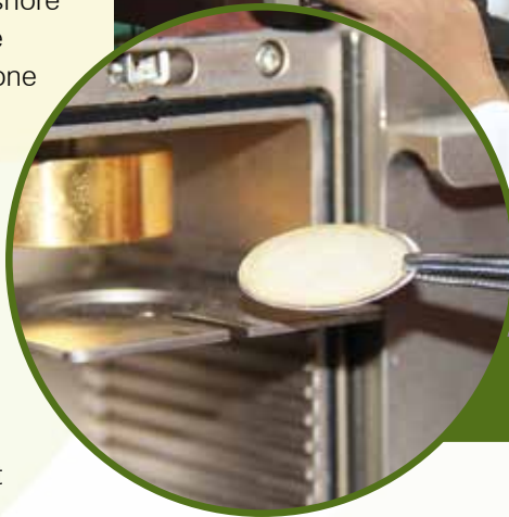
Measurement of lead-210 plated on silver disc (inset) using an alpha spectrometer
