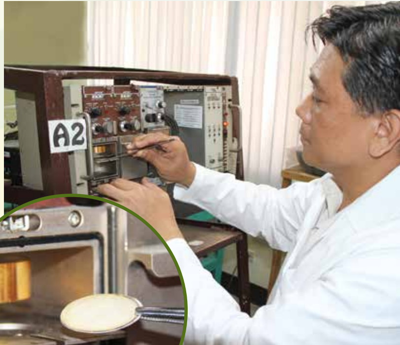
Measurement of lead-210 plated on silver disc (inset) using an alpha spectrometer
