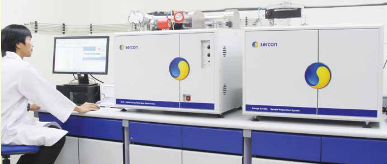
The new isotope ratio mass spectrometer, coupled with flash combustion and high temperature elemental analyzers, at the PNRI Soil Science and Crop Nutrition Research Laboratory for agriculture and environmental research
