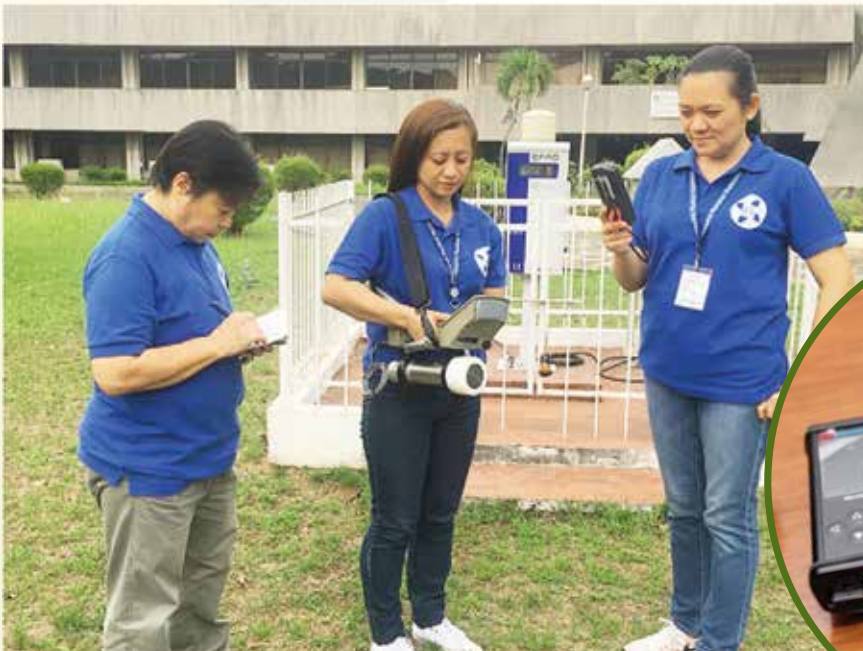
Monitoring in PNRI ground and its perimeter using a portable gamma dose rate meter (inset)
