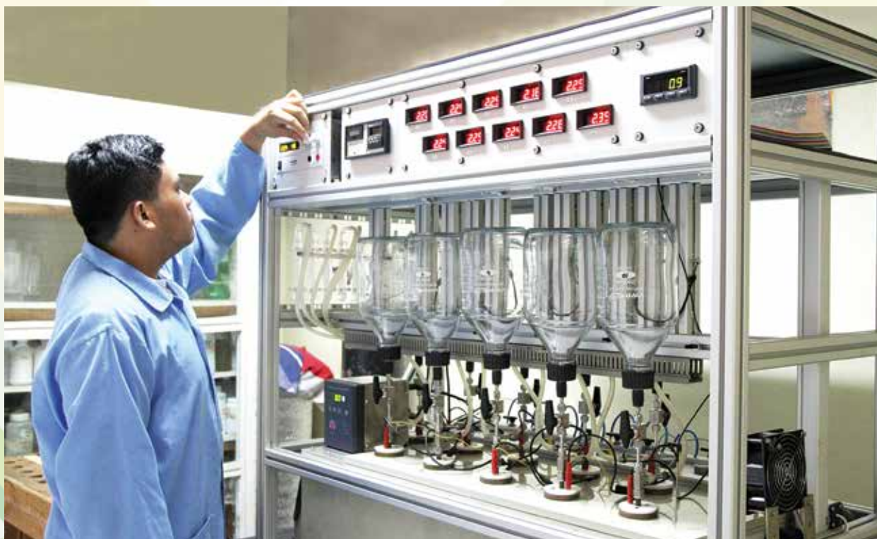
PNRI researcher uses the ultra low level tritium enrichment system for determining groundwater age
