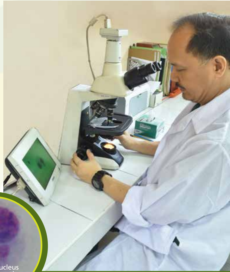
Microscopy for dicentric chromosome assay to monitor radiation exposure
