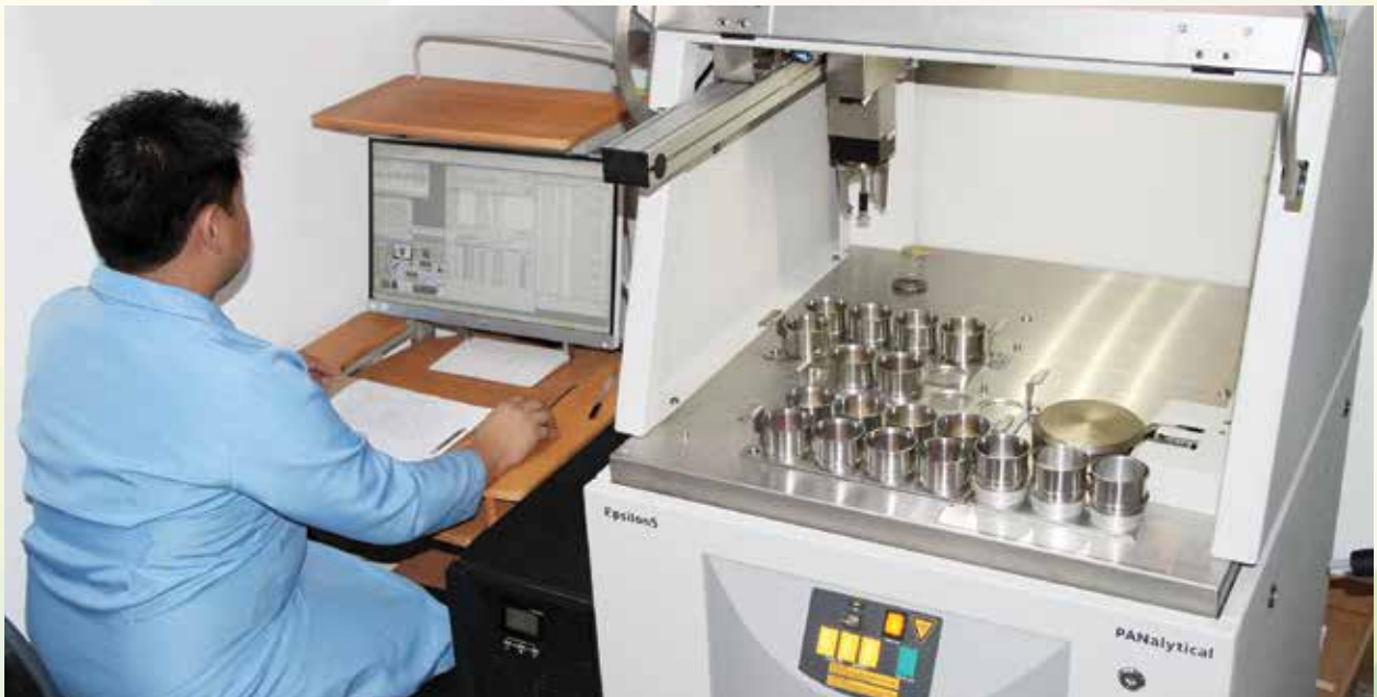
Analysis of air filter samples using the X-ray fluorescence spectrometer
