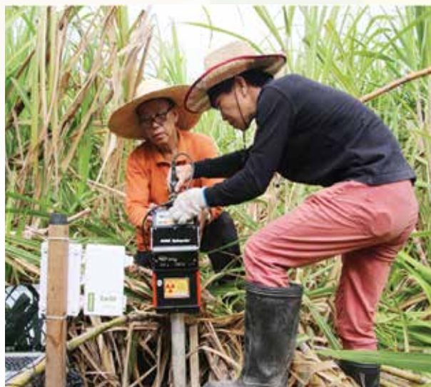
Gathering of data on soil water availability using soil moisture neutron probe as part of studies on increasing sugarcane productivity
