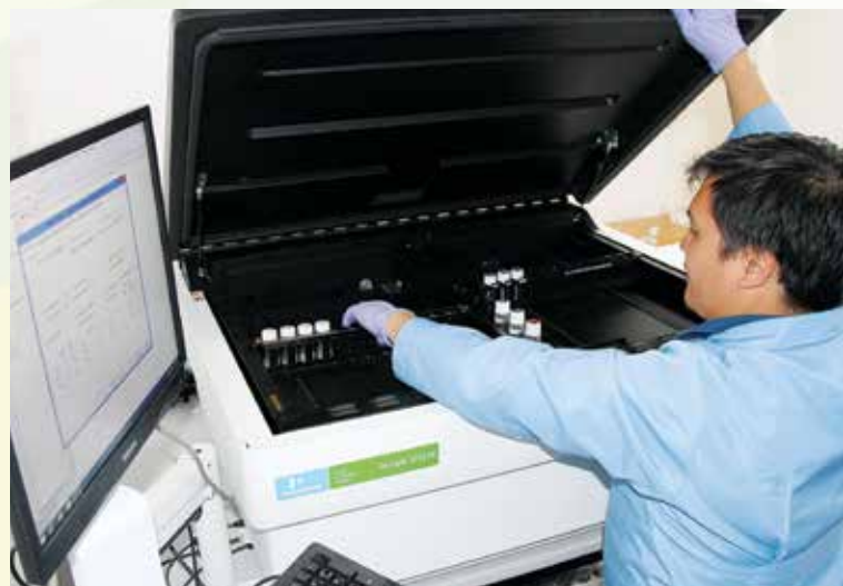
Analysis of synthetic acetic adulteration of vinegar samples using the liquid scintillation counter
