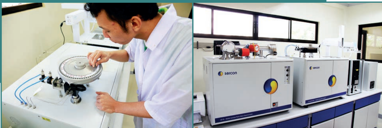
Researchers use an isotope ratio mass spectrometer to analyze the samples with isotope tracers, which are keys in studying nutrient use efficiency among crops.
