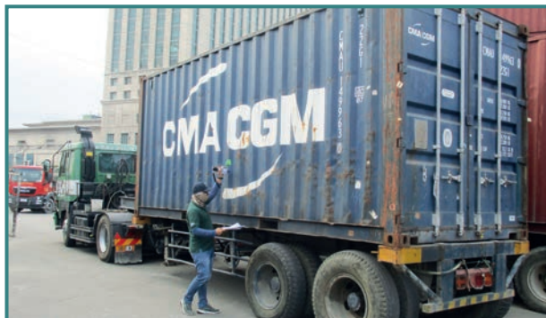
Cargo containers were monitored using handheld radiation equipment in the port of Cebu throughout 2019 as part of an IAEA research project on collecting radiation detection data for alarming containers
