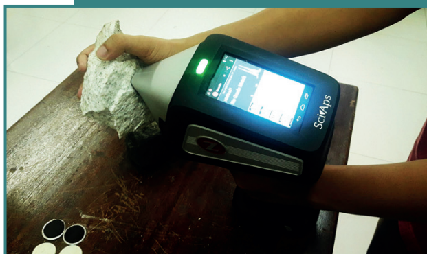
Analysis of a feldspar rock sample using laser induced breakdown spectroscopy analyzer
