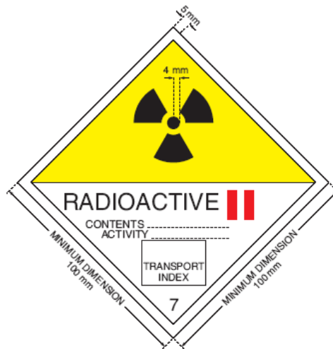
Figure 3. Category II-YELLOW label. The background color of the upper half of the label shall be yellow and the lower half white, the color of the trefoil and the printing shall be black, and the color of the category bars shall be red.
