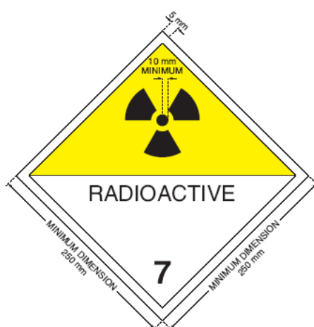
Figure 5. Placard. Minimum dimensions shall be as shown; when different dimensions are used, the relative proportions shall be maintained. The number '7' shall not be less than 25 mm high. The background color of the upper half of the placard shall be yellow and the lower half white, the color of the trefoil and the printing shall be black. The use of the word "RADIOACTIVE" in the bottom half is optional, to allow the alternative use of this placard to display the appropriate UN number for the consignment.
