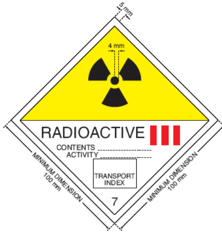
Figure 4. Category III-YELLOW label. The background color of the upper half of the label shall be yellow and the lower half white, the color of the trefoil and the printing shall be black, and the color of the category bars shall be red.
