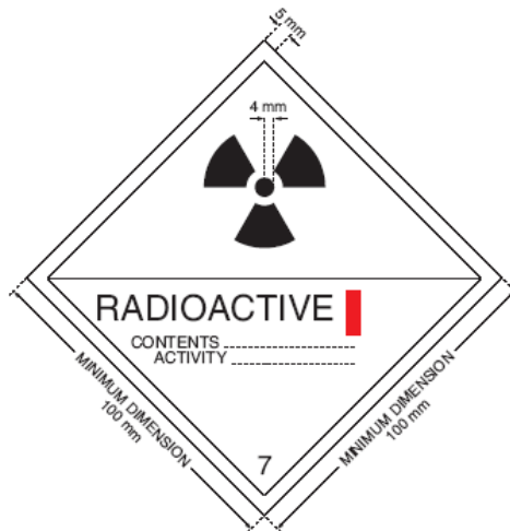
Figure 2. Category I-WHITE label. The background color of the label shall be white, the color of the trefoil and the printing shall be black, and the color of the category bar shall be red.
