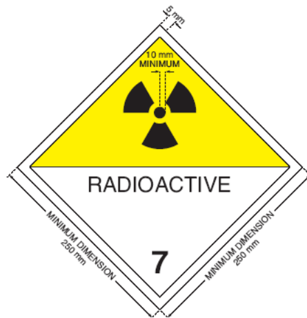
Figure 6. Placard. The number '7' shall not be less than 25 mm high. The background color of the upper half of the placard shall be yellow and of the lower half white, the color of the trefoil and the printing shall be black. The use of the word "RADIOACTIVE" in the bottom half is optional to allow the alternative use of this placard to display the appropriate United Nations number for the consignment.
