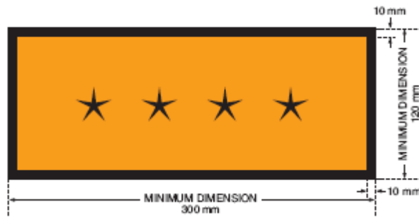
Figure 7. Placard for separate display of United Nations number. The background color of the placard shall be orange and the border and United Nations number shall be black. The symbol “****” denotes the space in which the appropriate United Nations number for radioactive material, as specified in Table VI, shall be displayed.
